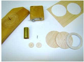
Turning back to the fuselage, I used 1/32<sup>nd</sup> inch balsa to sheet the forward part of the fuselage and cockpit area. Old Rhinebeck's Avro doesn't have traditional leather cockpit combing, but just thin strips of wood, so it was easy to just glue some balsa strips in place. One quarter inch balsa rings were cut and laminated to make up the cowl. I added some strips of styrene to represent the seams that is essential to the cowls look.
