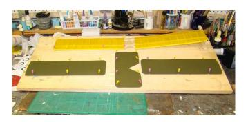
The wings panels were covered in tissue, shrunk with alcohol, and given two coats of highly thinned non-tauting nitrate dope with a bit of castor oil added to further help in avoiding warping of the light structure. The lower wings were then given a light coat of Tamiya olive drab paint.
