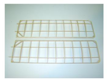
The rudder was constructed by soaking thin strips of balsa in water and ammonia overnight and then carefully pulled and taped around a form made from foamboard. When dry, I separated the parts, added glue, and returned them to the form to dry. The laminated part was then used to complete the rudder.
