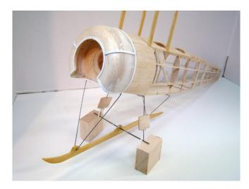
At this point, I gave all the balsa parts a couple coats of thinned nitrate dope and added brown Esaki tissue to the top and forward part of the fuselage.
