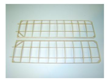
The rudder was constructed by soaking thin strips of balsa in water and ammonia overnight and then carefully pulled and taped around a form made from foamboard. When dry, I separated the parts, added glue, and returned them to the form to dry. The laminated part was then used to complete the rudder.
